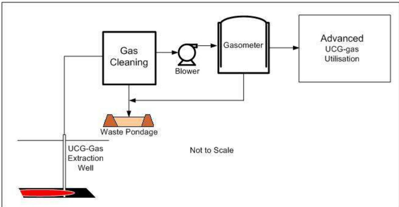
Figure 2. Syn-gas Flow, Well-head to Advanced Utilisation
