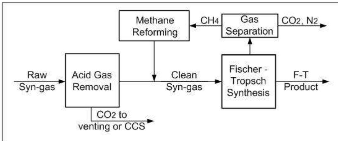
Figure 4a. Syn-gas Methane Reforming
